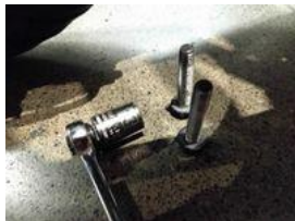
Nissin front caliper bolts 13mm hex 2014SR
