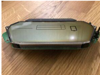
Instrument cluster board LCD drive pins
