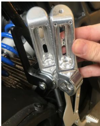
Sport Rider Footpegs vs Passenger Footpegs
