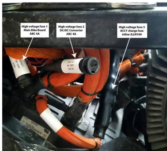
2016 Zero FX High Voltage Fuse Locations - Left Side
