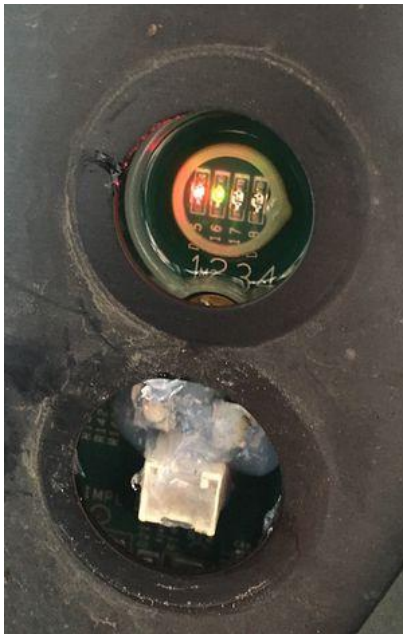
BMS indicator lights and reset windows on a 2016 DSR
