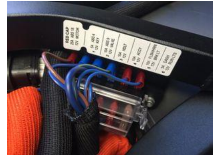
2015-2016 Fuse block (label inaccurate; rotated 180°)
